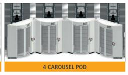
As the worker picks from one horizontal carousel in the pod, the other is pre-positioning the next pick. This minimizes worker downtime and dramatically increases throughput. Moreover, horizontal carousels arranged in pods offer great flexibility. With a simple software adjustment, the pods can be easily reconfigured to meet seasonal peak order times.
